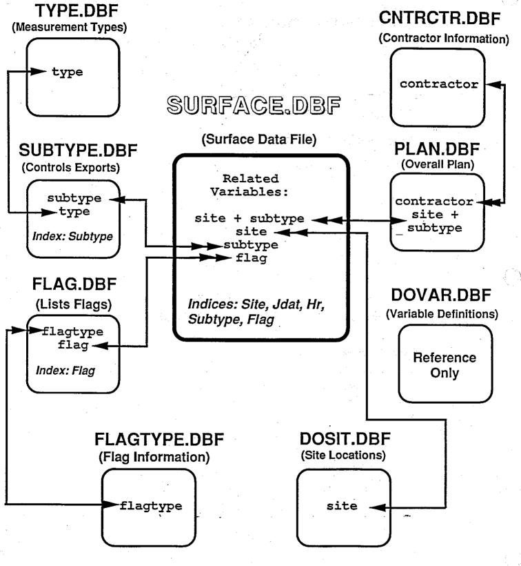
Figure 8 Date Flow For the SARMAP Surface Database
